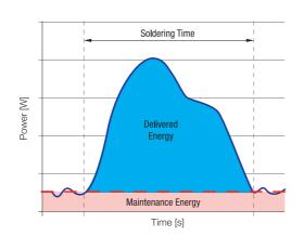
Soldering Assistant allows analyzing manual soldering processes and obtaining a qualification of these by comparing the soldering joints one by one.
